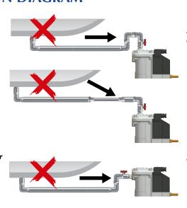
The feed pipe must be horizontal or ideally at a downwards slope (>1°).
